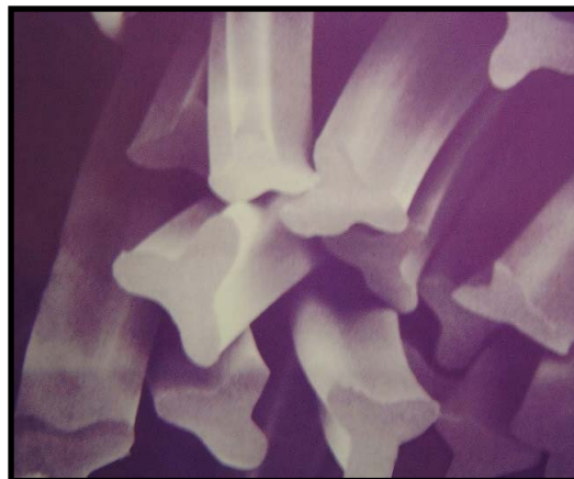
SEM image of multilobal / trilobal fibres
